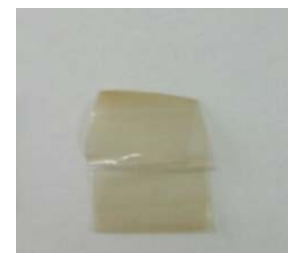
Composite containing max. 15 wt.% of Ag-Z
